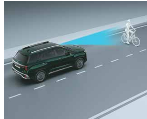
Forward Collision - Avoidance Assist - Cycle (FCA-Cyl)
