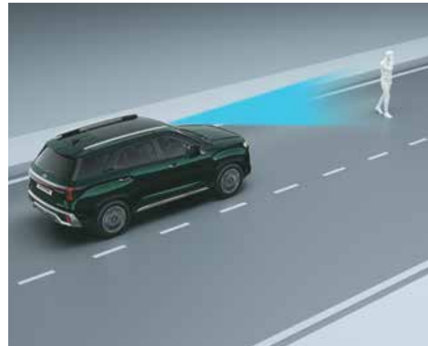
Forward Collision - Avoidance Assist - Pedestrian (FCA-Ped)
